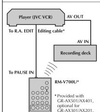
Using the RM-V700U, it is also possible to perform deck-to-deck Random Assemble Editing. The playback deck must be an R.A. Edit-capable JVC VCR. The recording deck can be...
